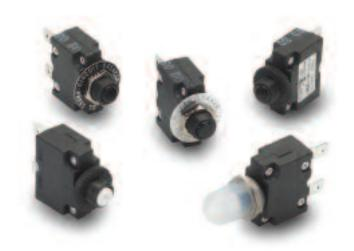
Rating: 3 to 20A, 125-250VAC, 32VDC Approvals: UL, CUL, CSA, TUV, CE UL1500/ISO8846 for ignition protection/marine Dielectric Strength: 2500 VAC/ 1 minute Interrupting capacity: 2500 amps Insulation Resistance: 100M ohms Operating Temperature: -10°C to 60°C
