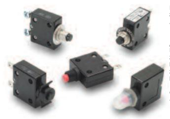
Rating: 3 to 60A, 125-250VAC, 32VDC Approvals: UL, CUL, CSA, TUV, CE UL1500/ISO8846 for ignition protection/marine Dielectric Strength: 2500 VAC/ 1 minute Interrupting capacity: 2500 amps Insulation Resistance: 100M ohms Operating Temperature: -10°C to 60°C
